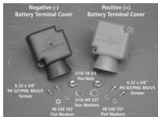
Figure 3-12 Battery Terminal Covers and Associated Hardware
