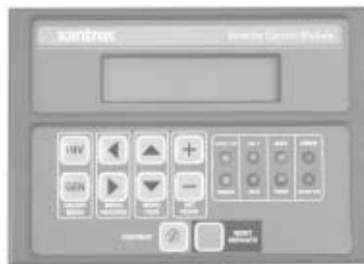
Figure 5-7 ICM Reset Defaults button
