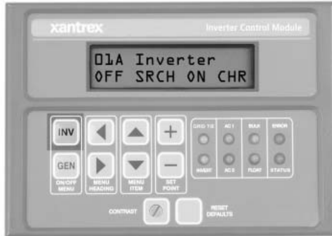
Figure 8-6 Inverter ON/OFF Display
