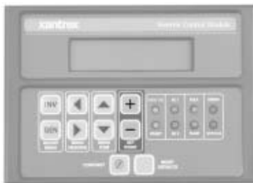
Figure 5-6 ICM Set Point Push-buttons
