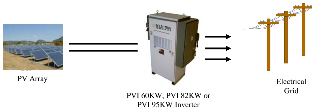
Fig. 1 Grid tied inverter application
