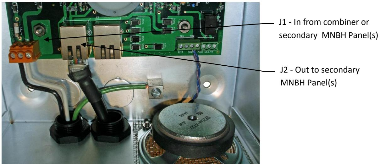
8. Connect the 600 volt UV rated CAT-5 control cable to the combiner at J1. Use a small amount of silicone grease on all cable ends to protect the connections.
